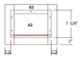
Fix the solid wood drawer box front with 5 screws at the places where the dots are. Assemble the drawer box and mount the soft close glides.
