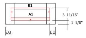
Fix the solid wood drawer box front with 3 screws at the places where the dots are. Assemble the drawer box and mount the soft close glides.
